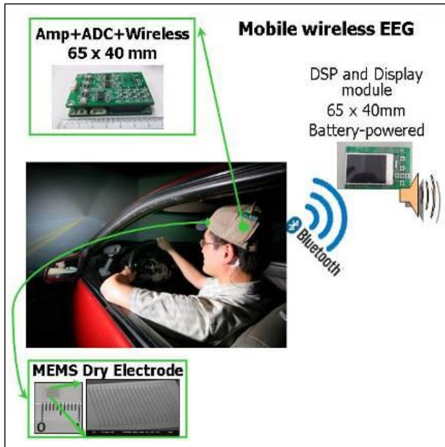
Figure 1. A wearable and wireless dry-electrode (WWD) EEG system that features dry MEMS EEG sensors (lower left), low-power signal acquisition, amplification and digitization, wireless telemetry (upper left), with online signal processing.
