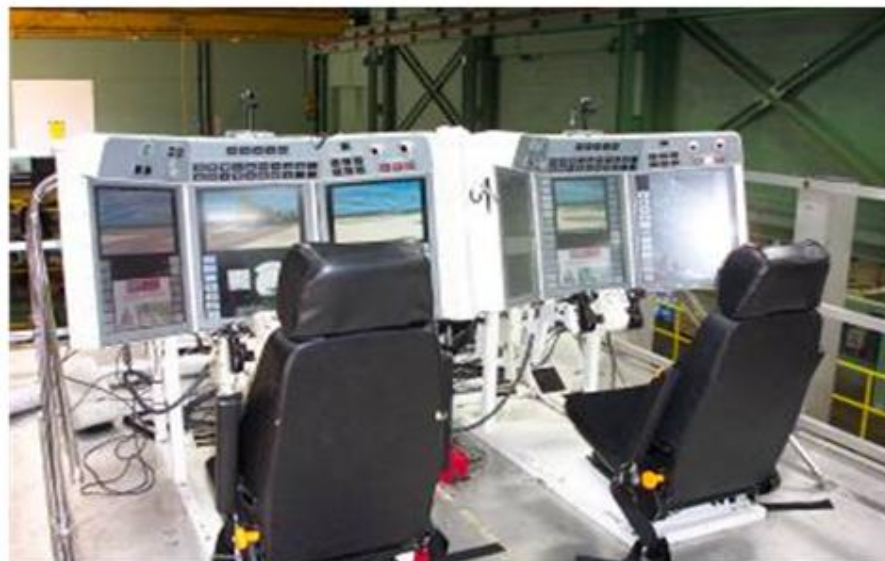
Figure 5. Example of crew station technology developed to optimize Soldier workload and provide the ability to conduct mission planning; route planning; reconnaissance, surveillance, and target acquisition (RSTA); and fire control capabilities. The crew station WMI software is fully configurable (up to six possible independent screens may be displayed simultaneously), portable (between crew stations), and interoperable. Here, two crew stations are shown as mounted on a large 6 DOF motion simulator located at TARDEC.
