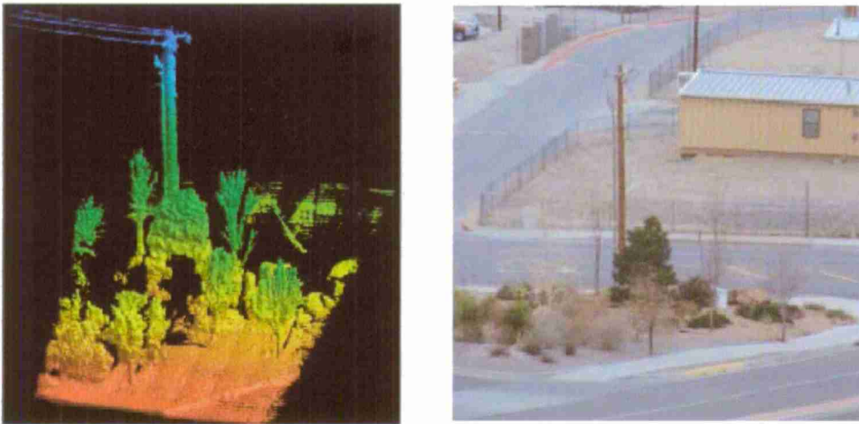
Figure 31. 3D image taken with a Spectrolab Gen-I 3D imaging camera. The picture is color coded with the range information. The right image is the same scene taken with a 2D vision camera (courtesy of Spectrolab).
