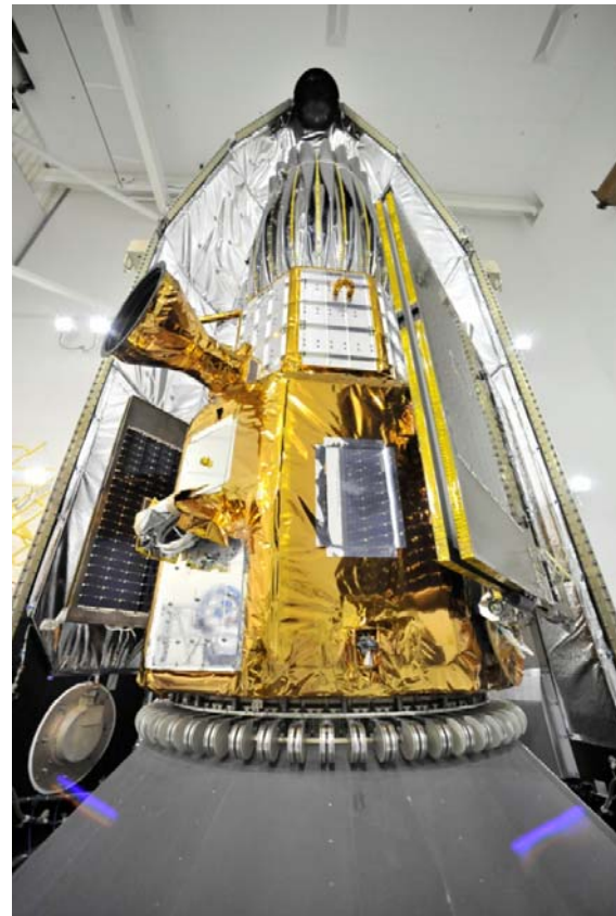
Figure 4. TacSat-4 During Fairing Encapsulation
