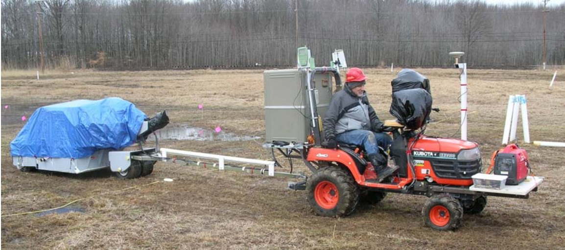
Figure 6. The ALLTEM surveying the APG Calibration Grid.
