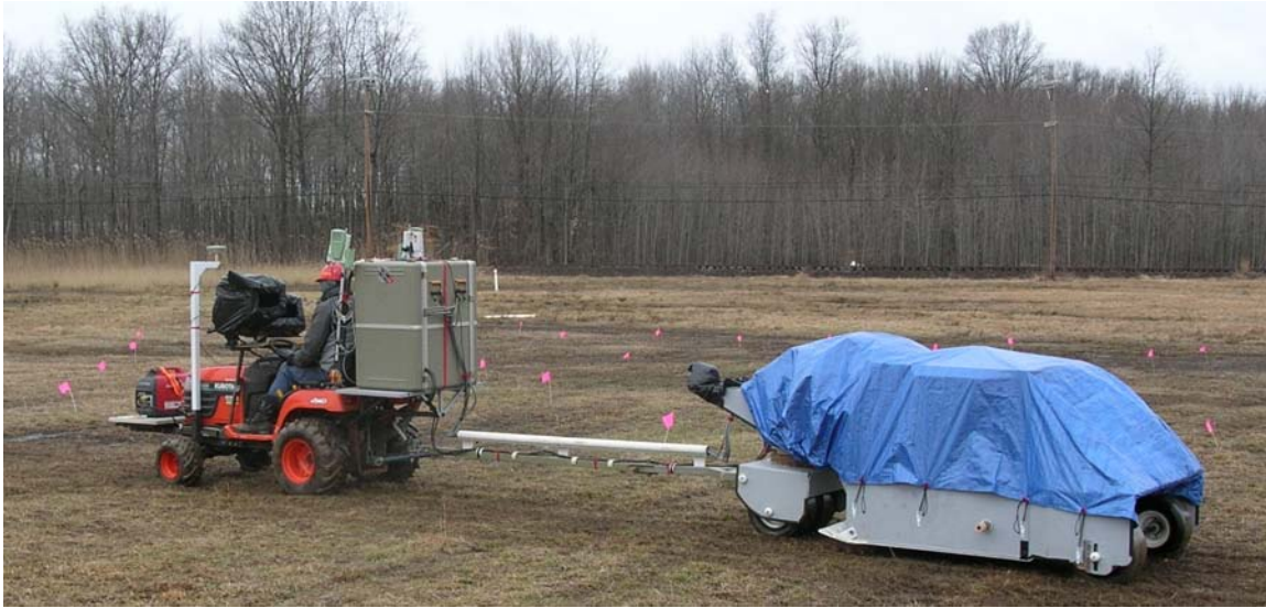
Figure 4. The ALLTEM surveying the APG Calibration Grid.
