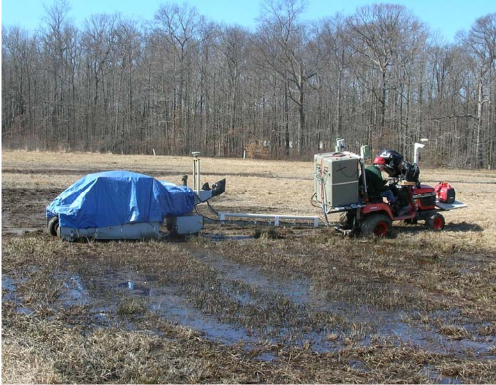
Figure 9. The ALLTEM surveying the APG Indirect Fire Area.
