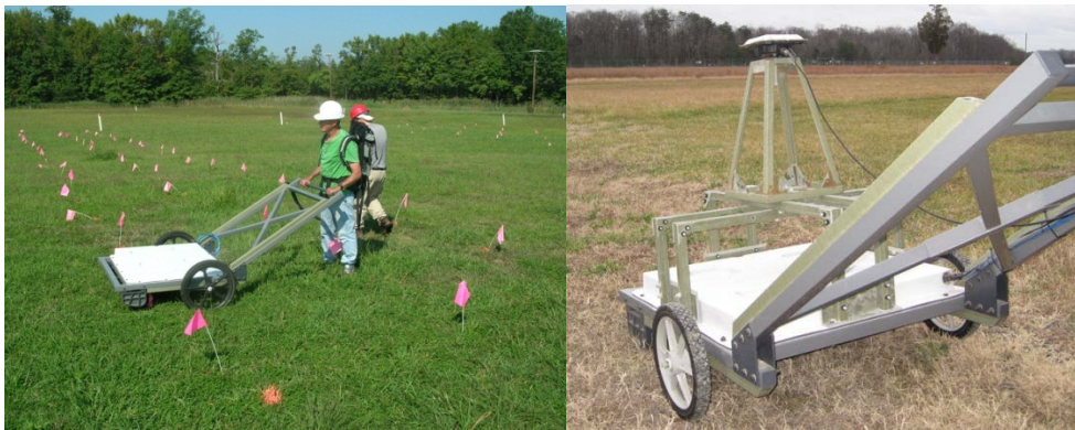
Figure 5-3 – The NRL TEMTADS Man-Portable 2x2 Cart (left) and TEMTADS MP 2x2 Cart with GPS Antenna Tripod (right)
