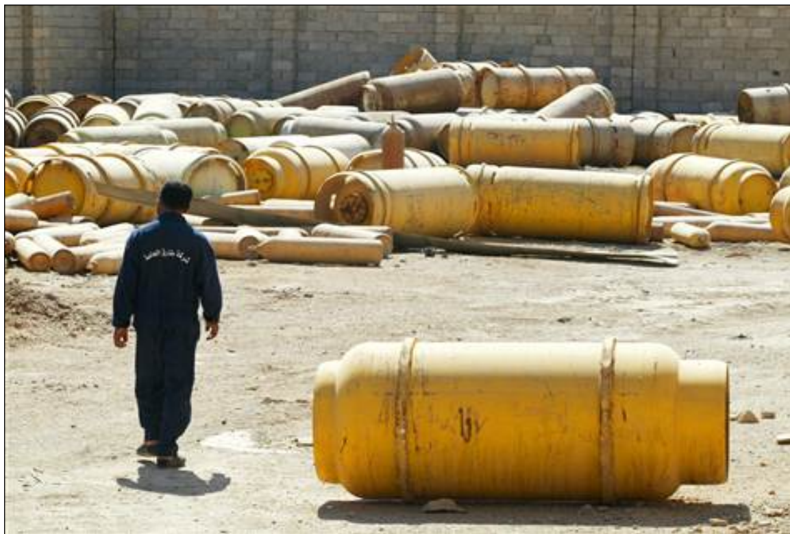
Figure 8: One-ton chlorine canisters unsecured at Fallujah II in October 2003. Note the presence of the two main types of one-ton container as well as 150lb cylinders.
