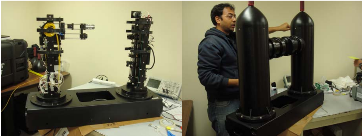
Figure 1. Internal electro-optical structure of the first in-situ HOLOCAM prototype (left panel). Pressure housings being assembled onto the HOLOCAM (right panel).
