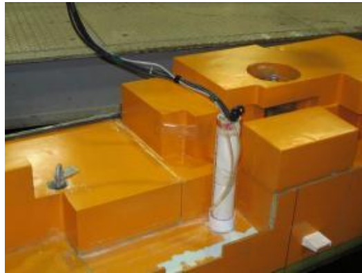
Figure 8. Model 5720 with chimney installed at the tether cable pass-through on the starboard side deck.
