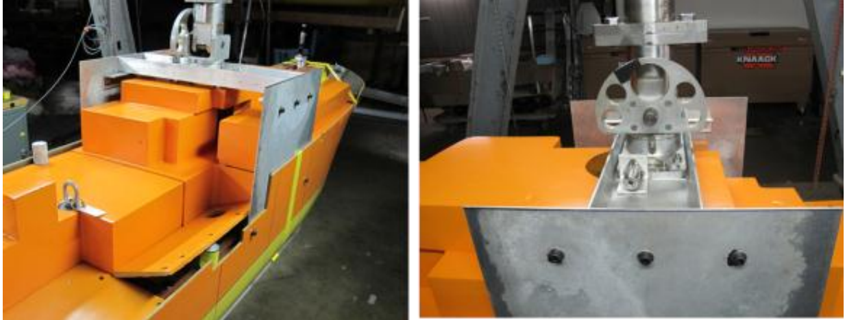
Figure 14. Mounting apparatus for model attachment to the pivot gear.
