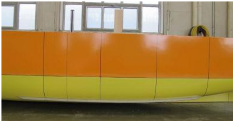
Figure 6. Model 5720 with port bilge keel shown, from forward to aft (left to right).
