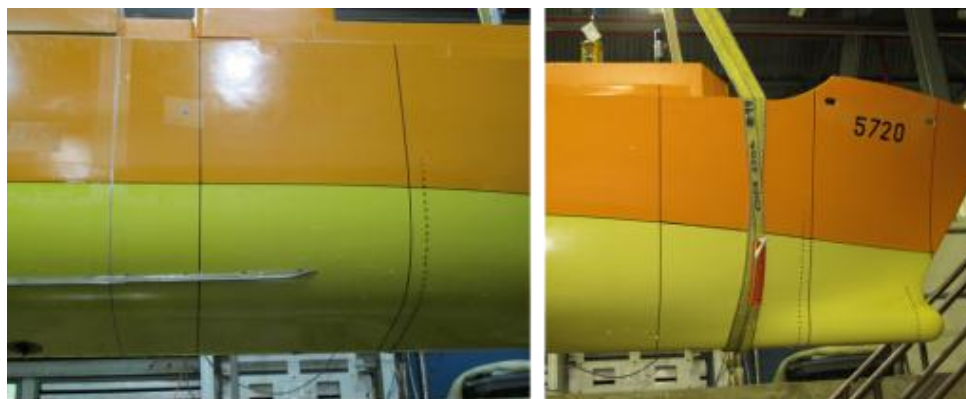
Figure 7. Model 5720 with turbulence stud spacing shown, forward of station 6 (left) and aft of station 2 (right).
