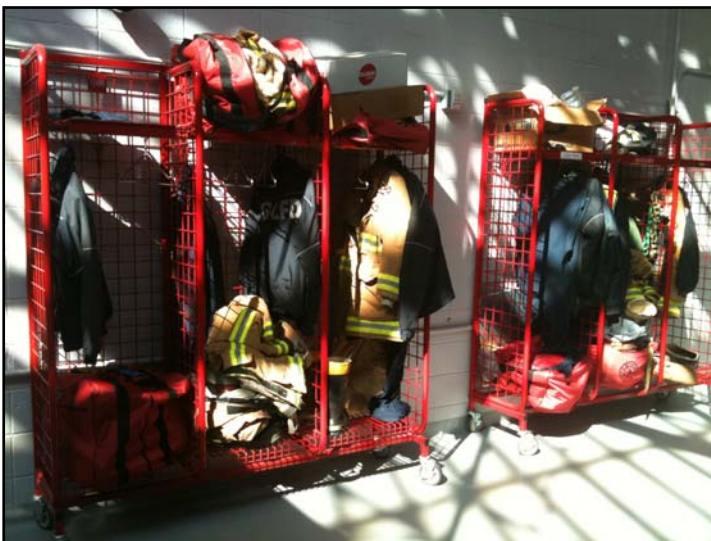
Figure 2. PPE in Stored in Open Bay and Exposed to Direct Sunlight After the Renovation
