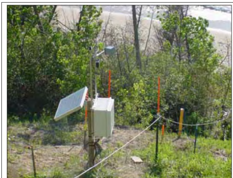
Figure 5. View from above of our site in a nearby control section of the bluff. Soil temperature, moisture, and resistivity instrument profiles in the bluff are marked by orange stakes, with solar panel, data logger, and web camera visible as a cluster in the foreground.
