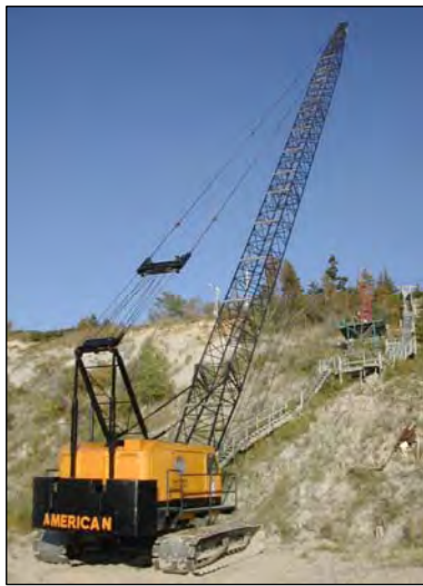
Figure 34. Green drilling platform and red drill at MPS suspended by 100-ft crane. Stairs have been rebuilt three times by property owners because of slope failures (photos after STS 2005).
