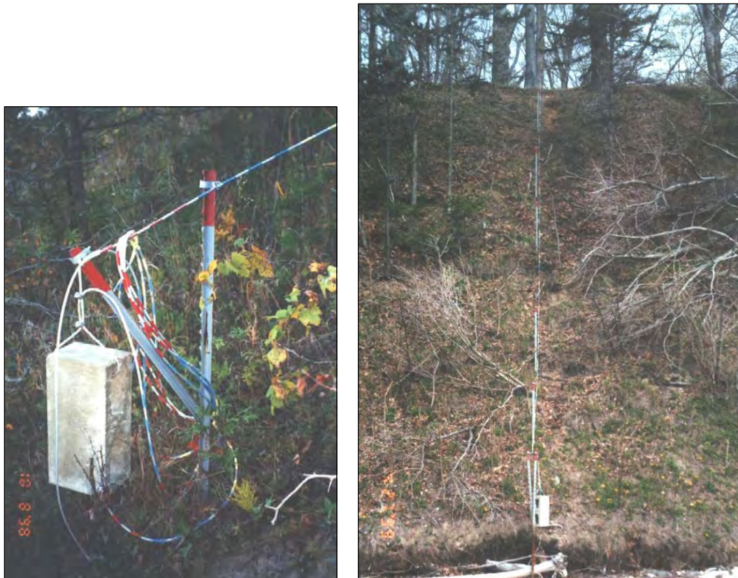
Figure 18. Last pole, left, of the calibrated pole-cable system and concrete anchor, and, right, calibrated cable system shortly after installation at 116 th Avenue.
