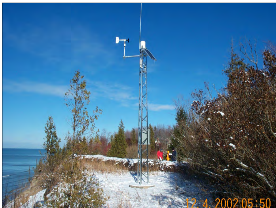
Figure 37. Solar-powered complete weather station at MPS. Identical system at 116th Avenue. Installed by WMU, STS, and USACE, Detroit District.
