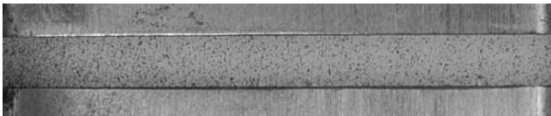
Figure 3. Side image showing the applied speckle and cropped raw image for compressive tests of the SC-15.
