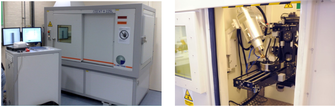
Figure 4. 6 - HMX ST scanner at \mu -VIS Centre [74], with a zoom of the internal configuration (right) where is possible to see the rotary stage and the X-ray source [75].
