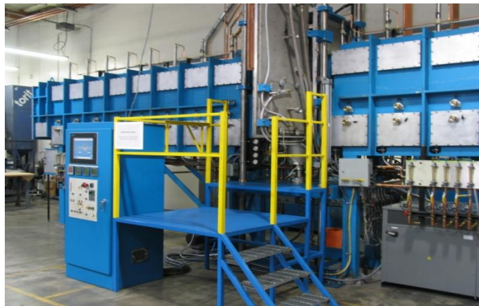
Hot pressing furnaces with multiple heating and cooling chambers, and a central hot pressing chamber
