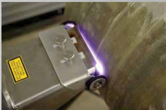
Laser ablation was optimized to remove coatings from submarine propulsion shafts and for other naval shipyard applications. (NMC photo)
