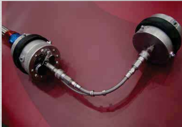
Improved construction processes for large diameter pipes in VCS, including the prototype pipe purging tool pictured, will save 8,500 labor-hours for a $590,000 savings per hull. (NMC photo)
