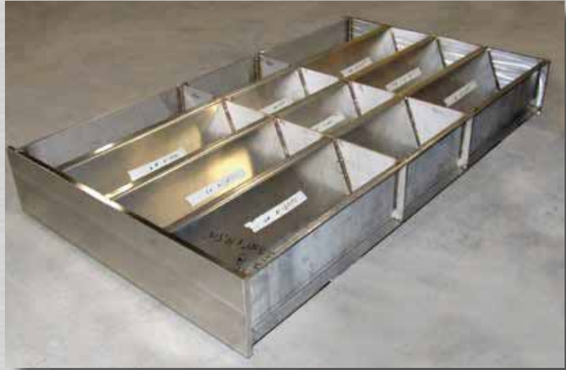
Various design for manufacturing improvements will reduce cost and weight for the LCS sliding doors. This photo shows a small-scale mockup that was constructed using welding procedures being investigated through this effort. (Applied Thermal Sciences photo)
