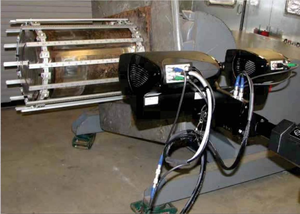
A white light scanning system will save the four naval shipyards significant costs in the inspection of main propulsion shaft connections on submarines and aircraft carriers. (NMC photo)
