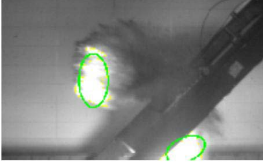
Figure 2.1 Video Frame with Entry and Exit Flashes and Fitted Ellipses [2]
