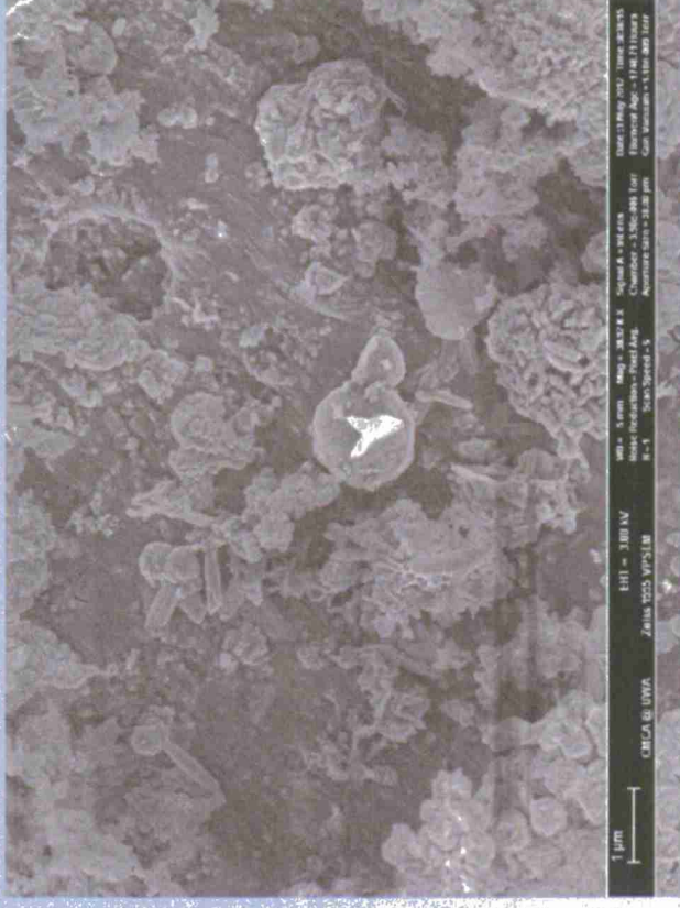
IRB: geothite, lepidocrocite, magnetite and hematite
