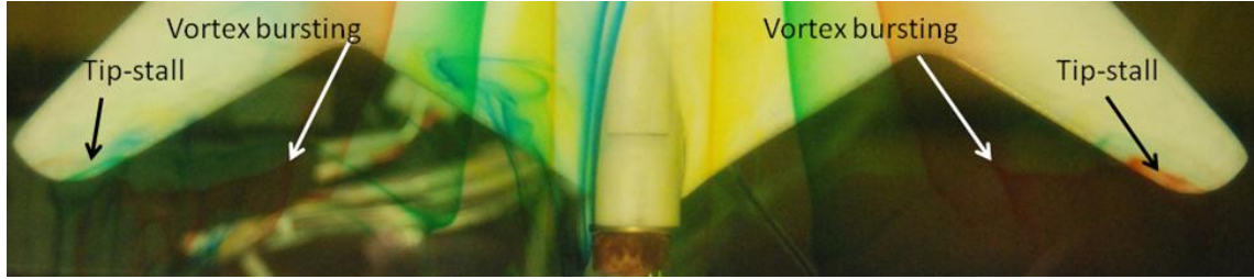
Figure 3. Close up of Tip-Stall from Trailing Edge Crank Vortex Bursting in Wake. Re = 4100 , \alpha = 6 degrees, steady flow. From [1].
