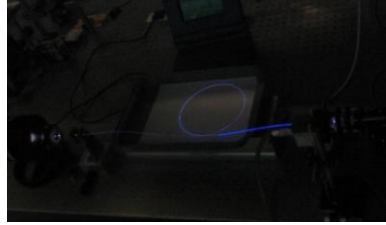
Figure 3.2. Tm-doped fiber laser using free space coupling of pump.
