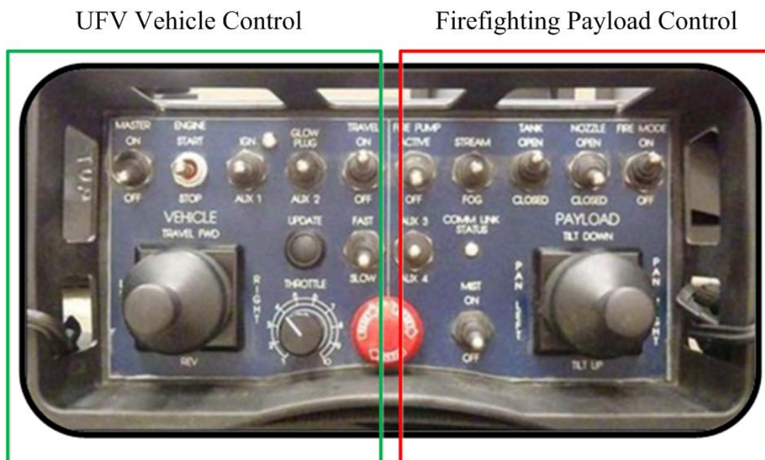
Figure A-2. Fire Defender Miratron Controller
