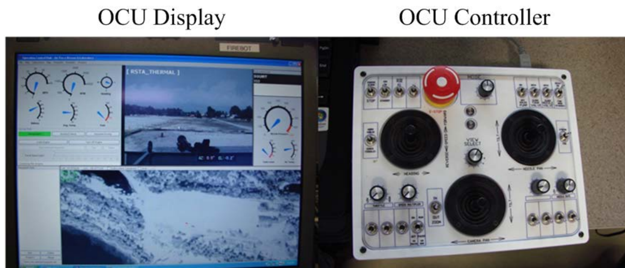
Figure B-1. Upgraded Fire Defender Operator Control Unit (OCU) Controller and Display
