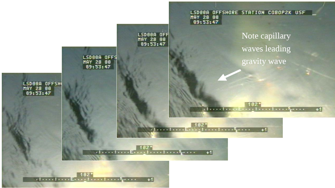
Figure 1. Video sequence from underneath the sea surface (0.25 m depth) showing wave train development. Note the group of capillary waves leading a gravity wave.
