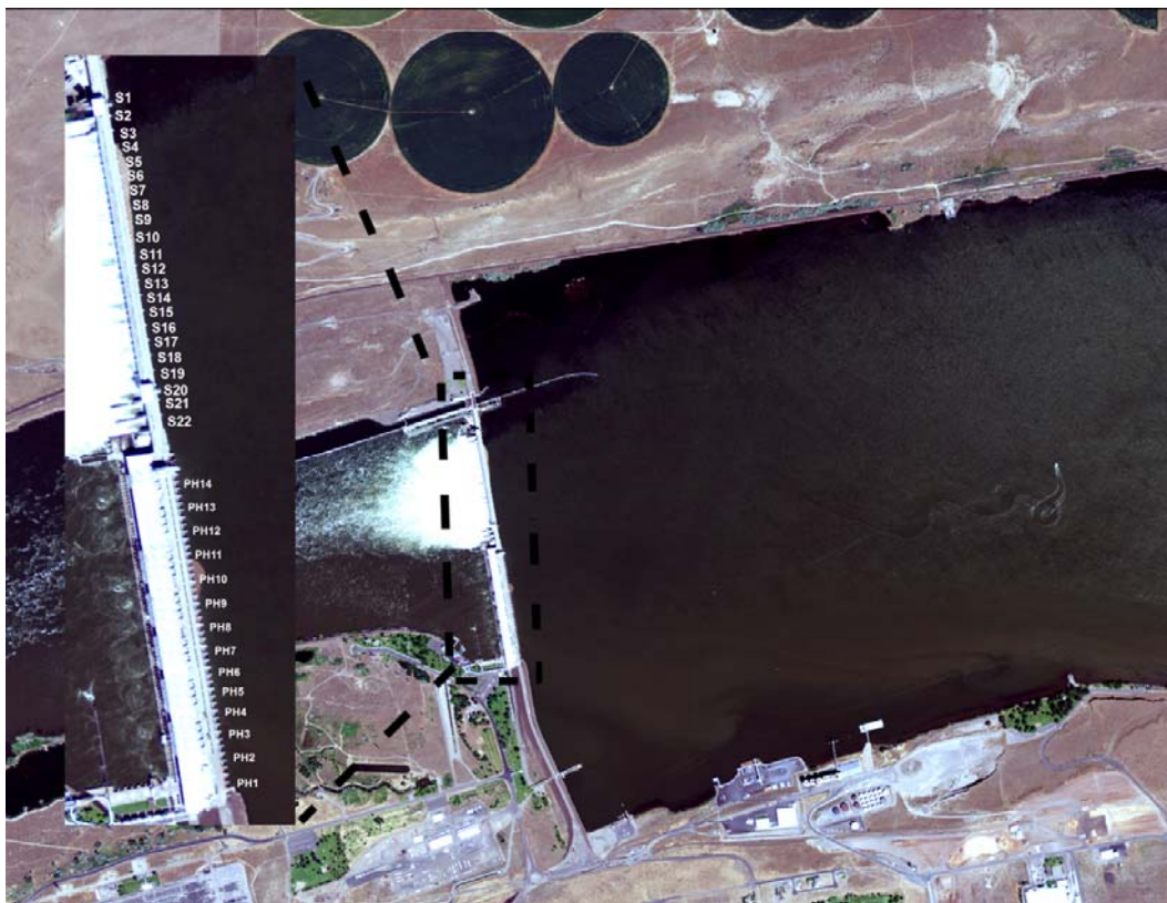
Figure 1. Plan view of McNary Dam Forebay showing the spillbays and powerhouse units.
