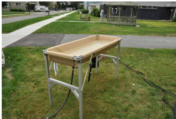
Figure 1-3. Arm Immersion Cooling Device. To use, Soldiers place their forearms in the cool water, covering the area from the fingers to the elbow.
