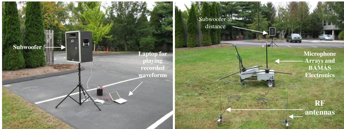
Figure 15: Preliminary acoustic test of both BAMAS sensors.
