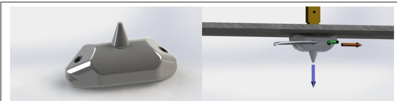
Fig. 6. Computer model of earlier tag model AM-240A (left image) and force sign convention used for reporting the results (right image). Flow is from left to right. The blue, red, and green arrows indicate, respectively, positive lift drag and side forces. The clear arrow indicates positive rotation angle.
