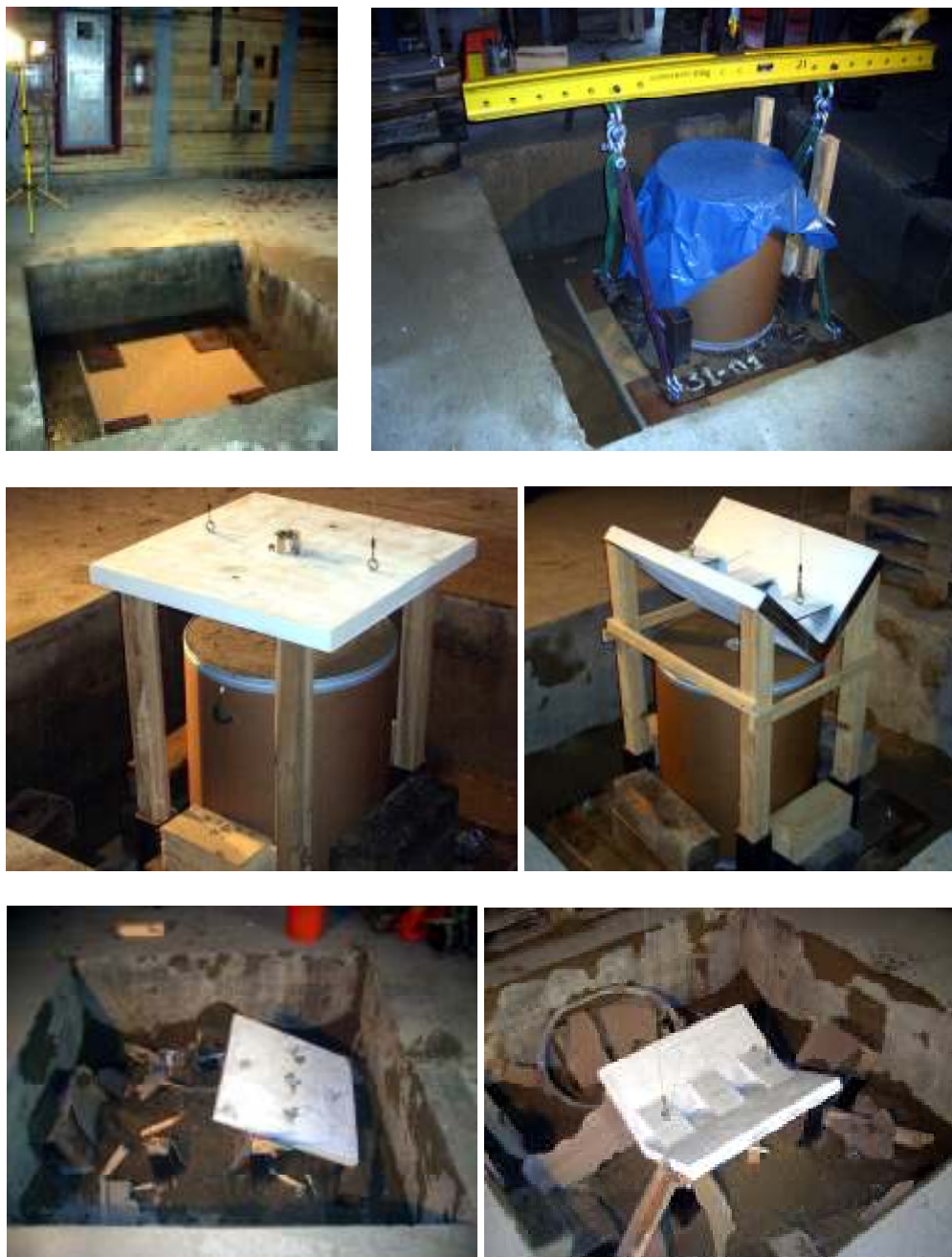
Figure 10. From top to bottom row: setup inside the blast laboratory; position of plates before initiation; post-test photographs.
