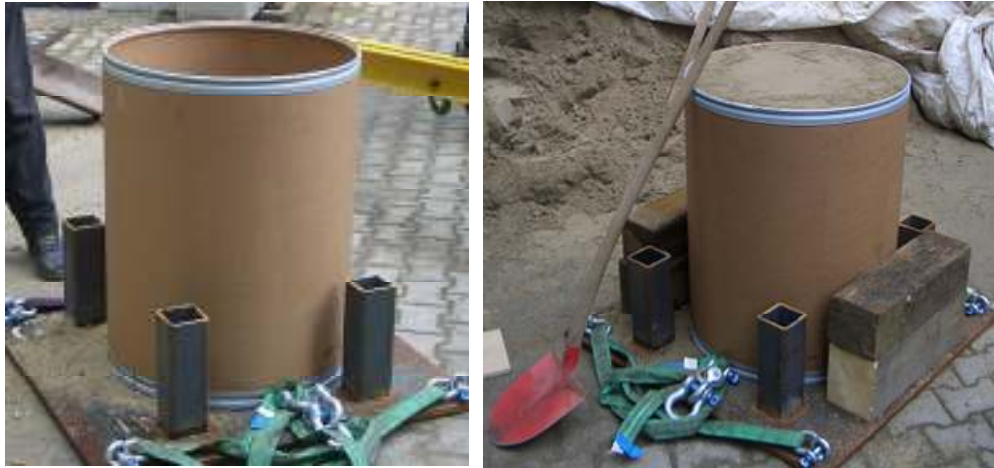
Figure 4. Cardboard barrel (on steel support) used for the experiments.
