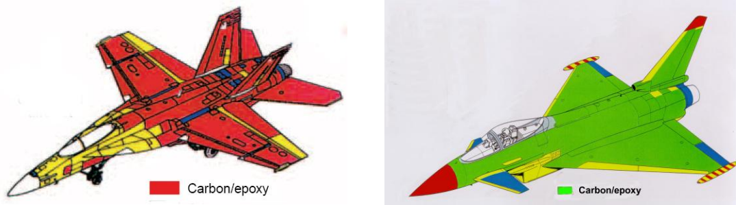
Figure 1-0-2: Outer Surface Material Usage of Modern Fighter Aircrafts
