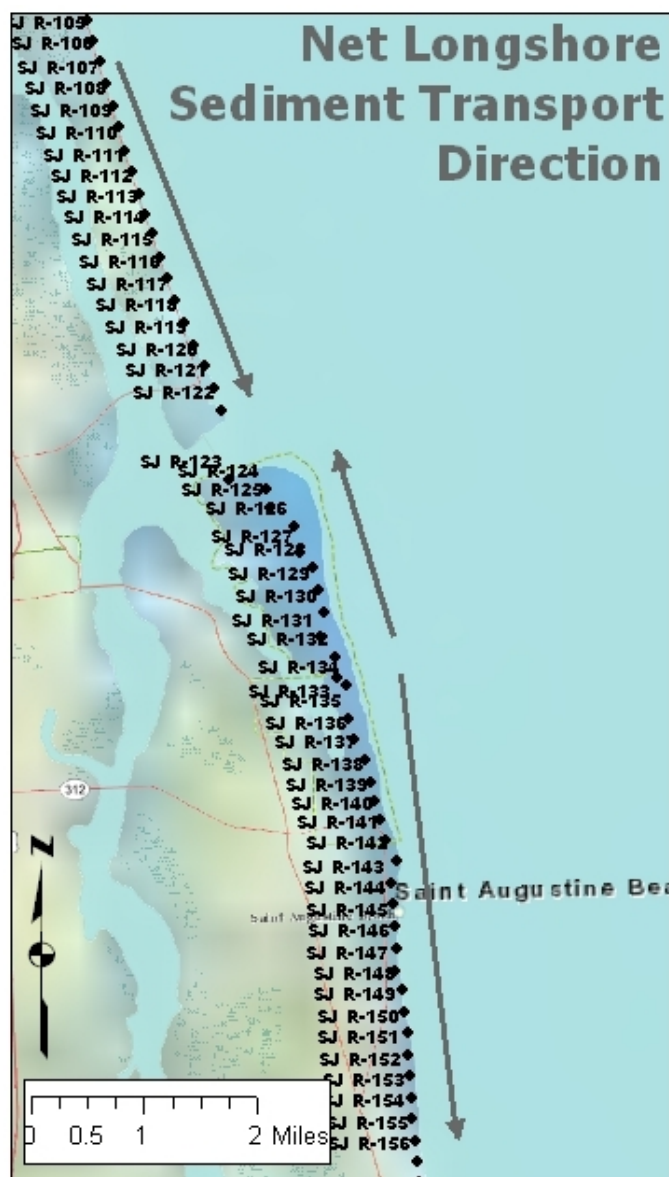
Figure 6. General net longshore sediment transport directions in the vicinity of the inlet.
