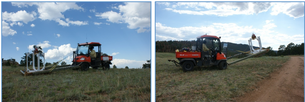
Figure 1. The SKY3D MetalMapper. The SKY3D MetalMapper extended in survey mode (LEFT) and elevated in transport mode (RIGHT).
