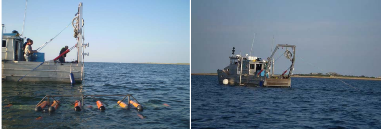
Figure 9. MGA towing operation: preparation (left), surveying (right).
