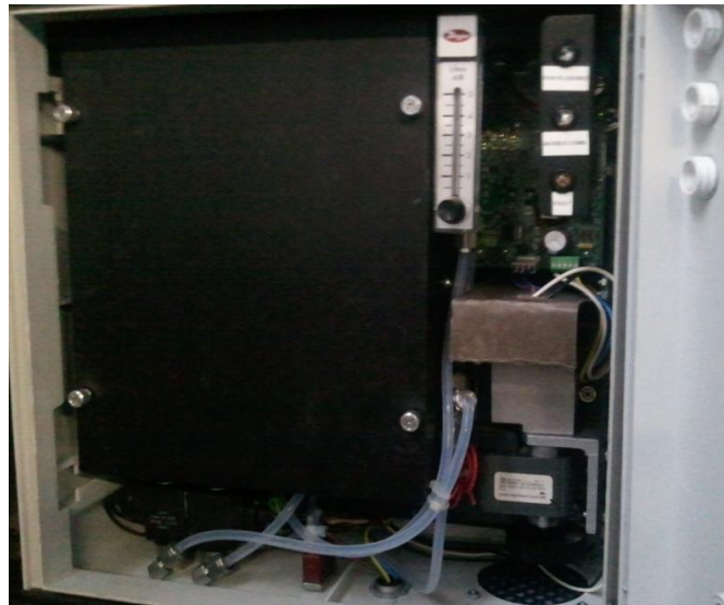
Figure 9. The prototype multisensor box used for CO/O 2 trim closed loop control.
