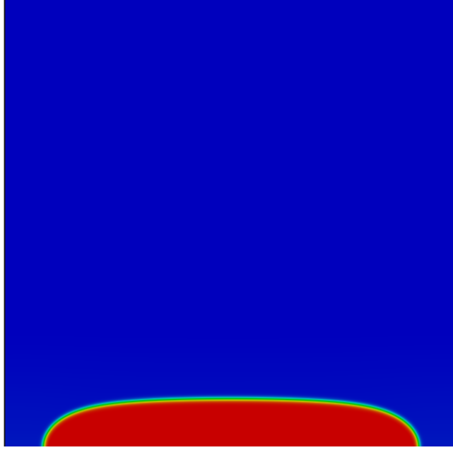
Figure 20: Solution of liquid droplet on solid surface at t = 20.0 with |\mathbf{f}| = \mathbb{B}_0/\text{We} = 5.0 \times 10^{-2} .
