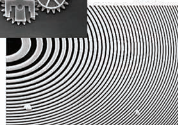
Zone plate X-ray "lens" Outermost ring spacing ~35 nm
