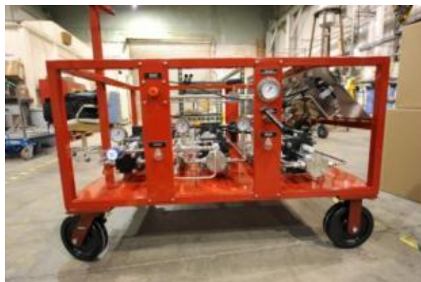
Figure 19. Gas Booster System for Gas Transfer
