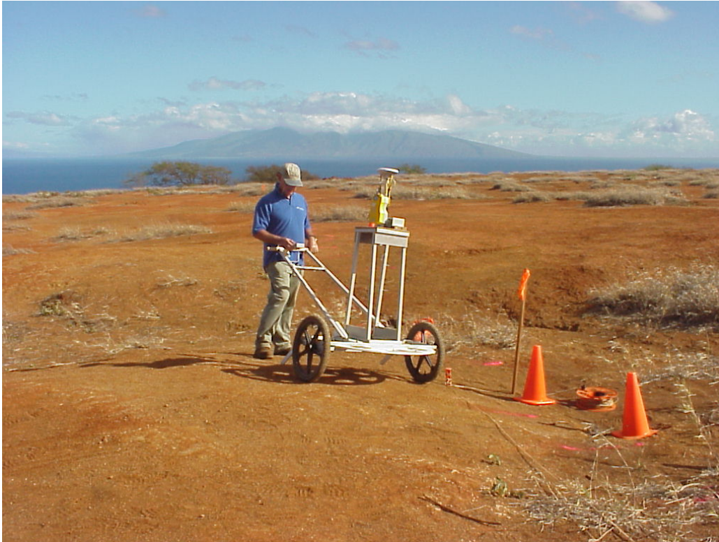
Figure 6.36: A photo of Alex Oren from Geophex Ltd. collecting data at the Kaho‘olawe UXO test site. Data were collected with cart mounted version of the GEM-3. A 1 m circular transmitter loop was used for the demonstration.
