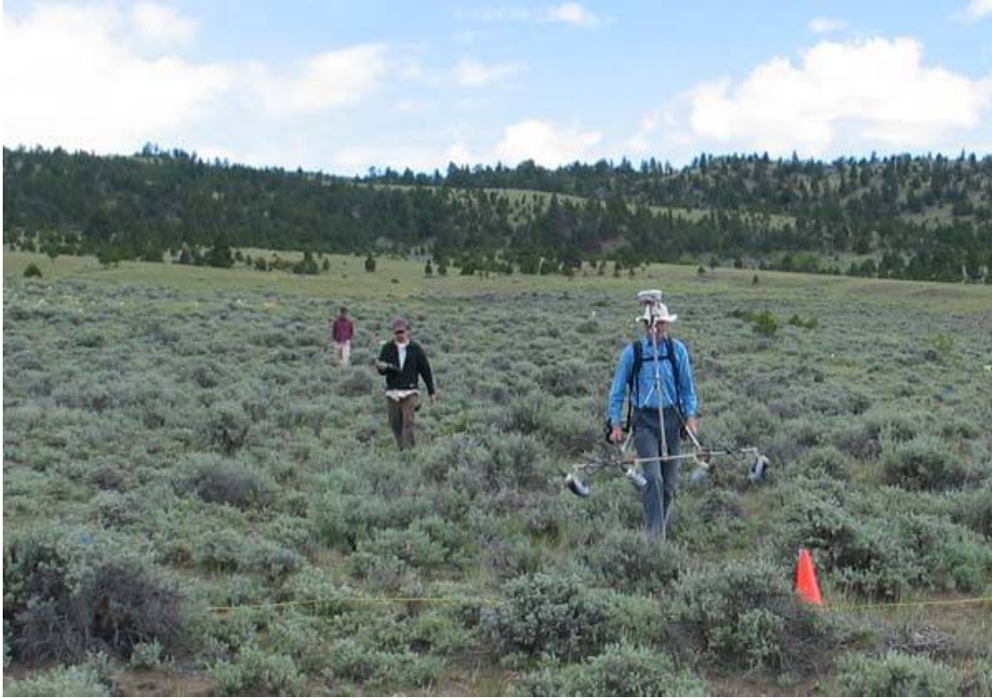
Figure 2.18: Magnetics data collection using the Sky Research magnetometer array at Chevalier Ranch, Montana.
