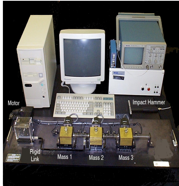
Figure 1. Experimental Adaptive Vibration Isolation Testbed
