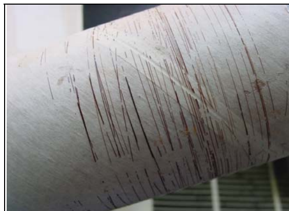
Figure 77. Photograph showing sticking of Ace_SKL to the roll surface due to insufficient evaporation of acetone.
