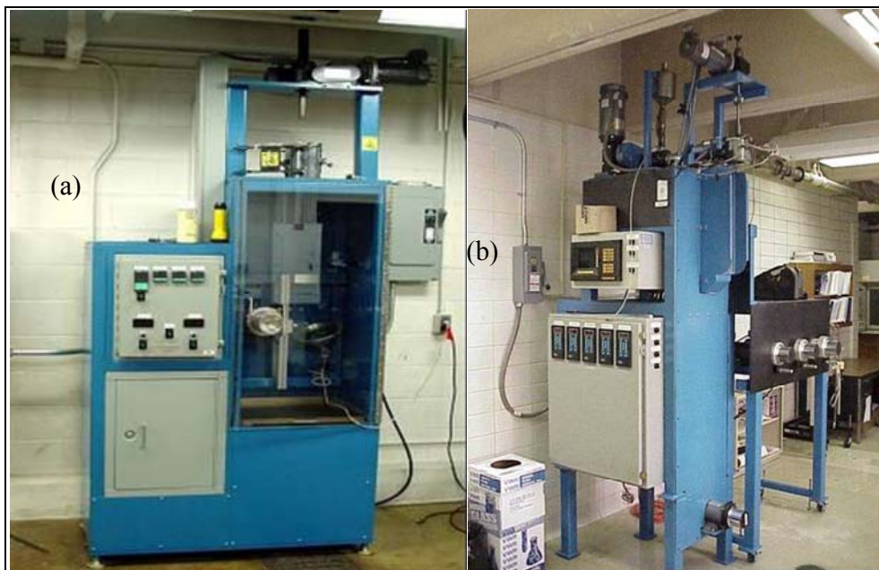
Figure 16. (a) Batch spinning unit for samples up to 100 g and (b) continuous fiber spinning unit for large-scale laboratory production of fibers at rates up to 5 kg/day.
