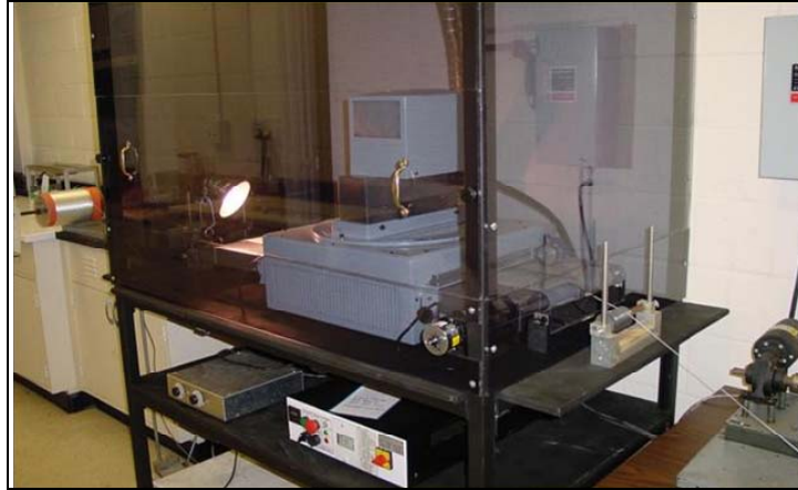
Figure 17. Custom-built, 5-kW UV irradiation chamber for batch or continuous irradiation of carbon precursor fibers.
