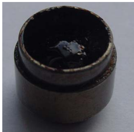
Figure 49. A consolidated melt resulting from softening point test on Ace_SKL (ball removed).
