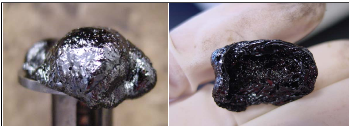
Figure 56. Foamed soda lignin after heating to 250 °C.
