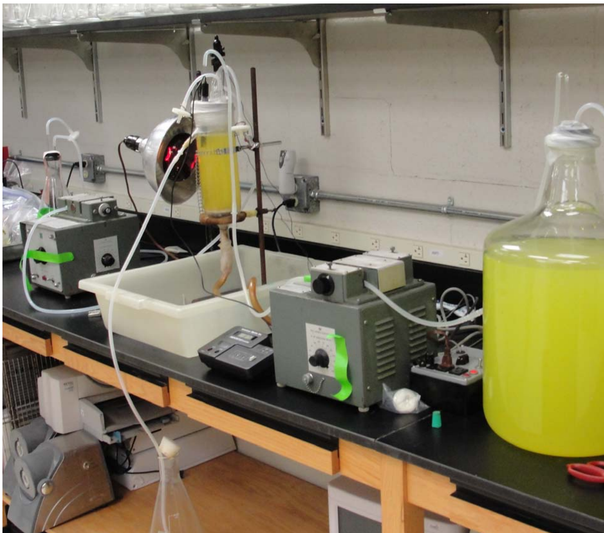
Figure 28. Chemostat assembled for lignolytic microorganism isolation.
