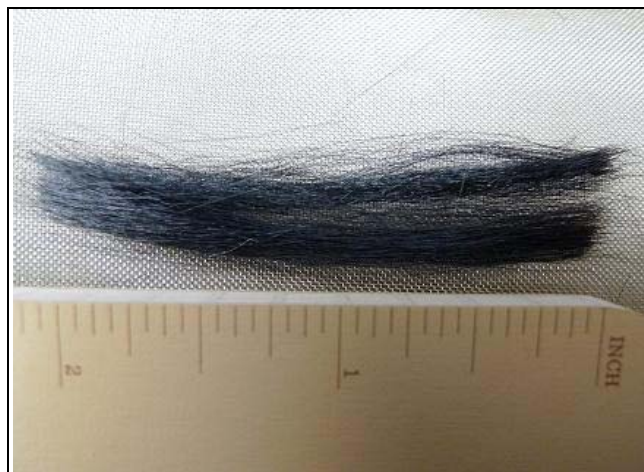
Figure 79. Oxidized, solution-spun Ace_SKL with low concentration of acetate groups.
