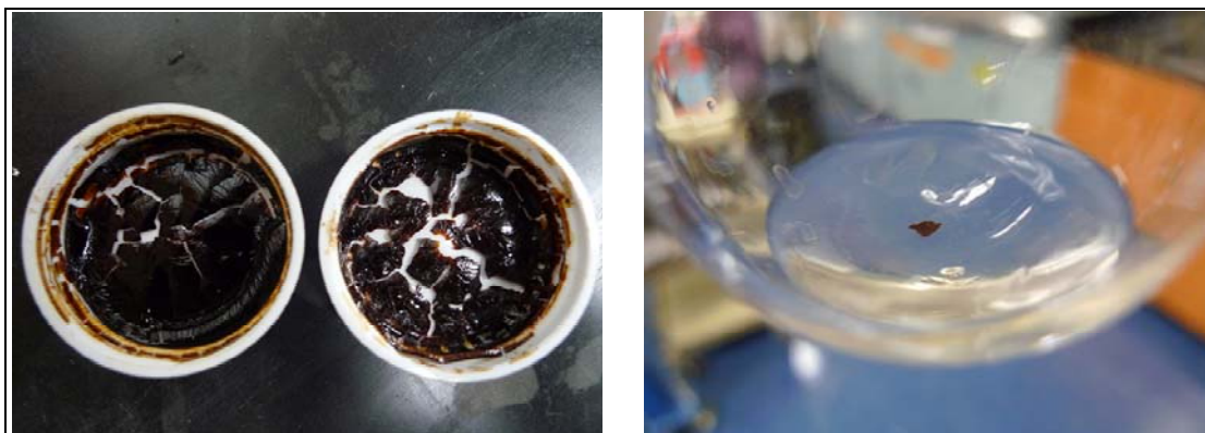
Figure 67. Left: Film chips made from methacrylated SKL. Right: film chips of methacrylated SKL tested with acetone.
