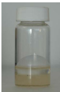
Figure 140. Photograph showing insolubility of UPE1/styrene (70/30).
