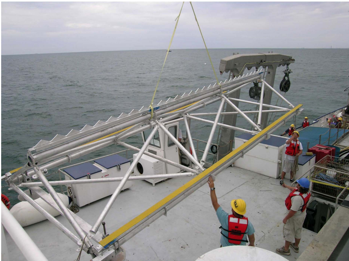
Figure 1. One 7-m rail section being prepared for deployment. Four sections were joined together on the bottom to form the full rail system.
