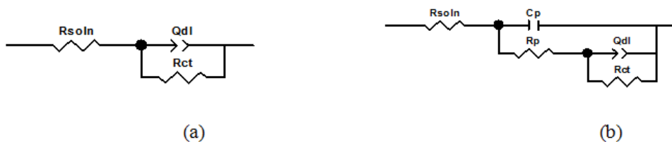
Figure 91. Equivalent circuits used to fit EIS data: (a) one time constant and (b) two time constants.
