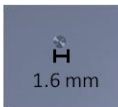
Figure 116. Representative artificial defect ( \sim 1.6 \text{ mm} i.d.) machined into field areas of panels to provide a controlled test area.
