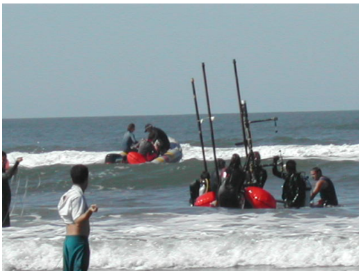
Deploying instrumented tower in the surf-zone
