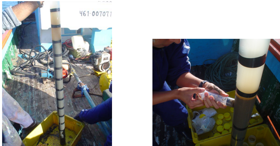
Figure 8: Core taken at 12m station, and sampling procedure.
