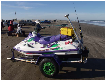
Instrumented Jet-ski for nearshore surveying
