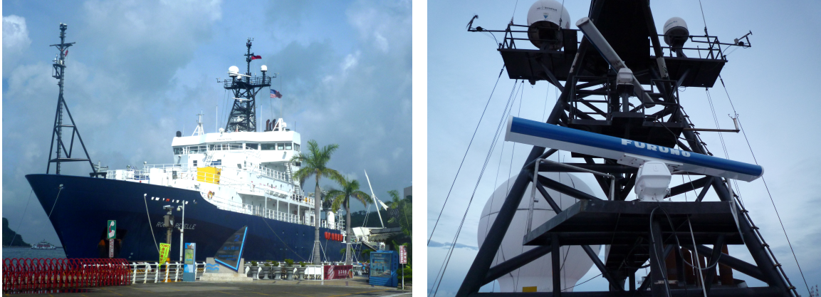
Figure 3.1: Pictures of R/V Roger Revelle in Kaohsiung harbor, taken on June 16, 2010, and of the ship's main mast with the X-band radar antennas for wind retrieval (bottom) and navigation (top) [photo credit: Wolfgang Hüneburg, OceanWaveS GmbH].
