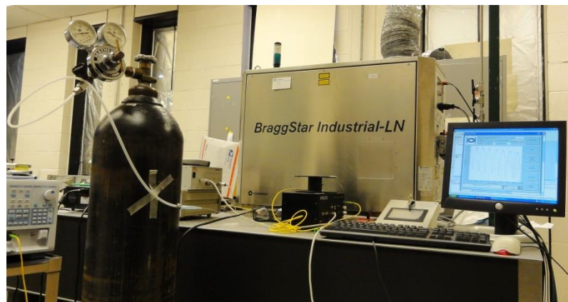
Figure 4.1 Measurement setup, includes air pressure source, Si125 interrogator, and computer
