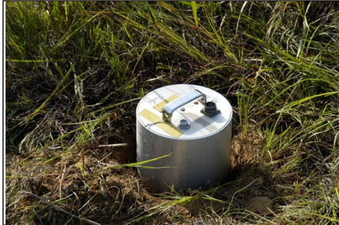
Figure 3-51a. Triaxial Geophone: Geophone Placement, Partly Embedded Prior to Backfilling
