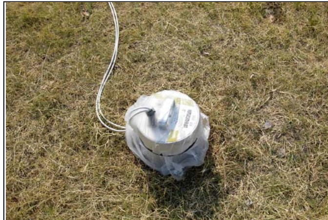
Figure 3-51b. Triaxial Geophone: Geophone in Use, Wiring Harness Connected and Covered with Plastic Bag
