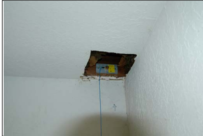
Figure 3-53 Accelerometer Placement on Top Plate (Through Ceiling), Building 6961B
