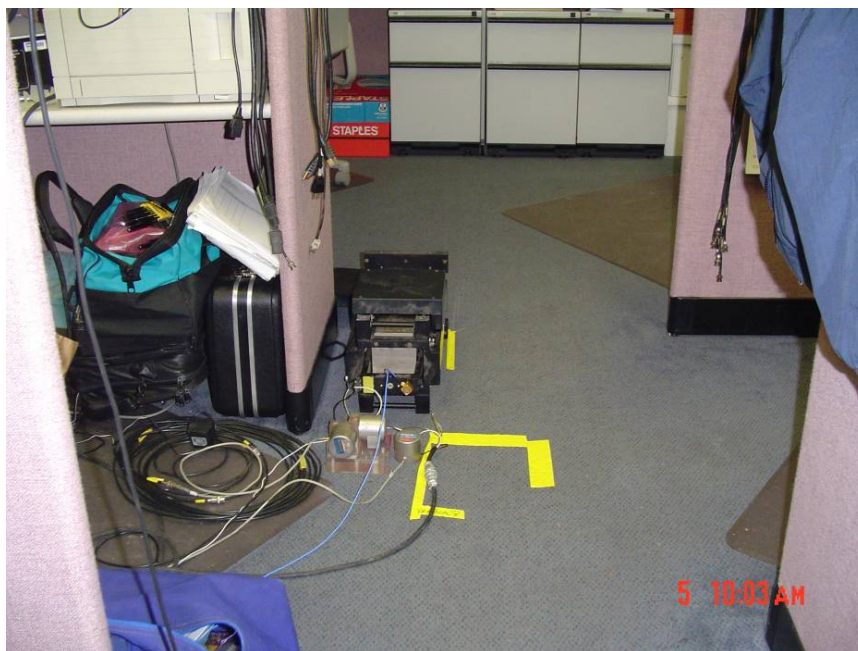
Figure 3-31. APG Building 2006: View of the Horizontal Shaker Setup at Location 3 (floor level) Near the Interior Front Wall, in the East Half (to right is S) (The shaker is aligned to the east-west direction)
