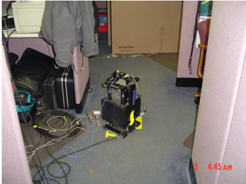
Figure 3-30. APG Building 2006: Vertical Shaker Setup at Location 3 (floor level) Near the Interior Front Wall, in the East Half (to right is S)
