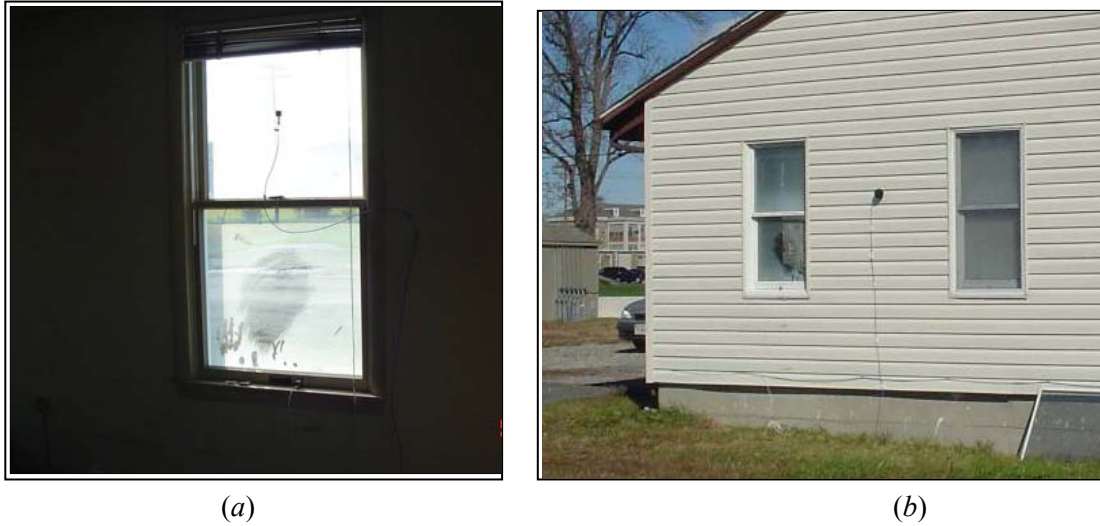
Figure 3-42. APG Building 4031: (a) Interior View of Accelerometers Mounted on the Window and Window Sill; (b) Exterior View of the South Wall with Accelerometer on Window Sill and Wall Microphone
