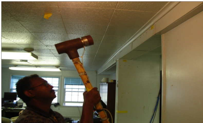
Figure 3-74. MCAAP Building 97A: Instrumented Hammer Testing
