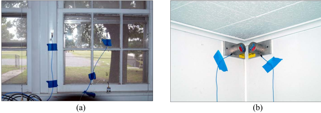
Figure 3-73. MCAAP Building 97A: (a) Instrumented Window; (b) Accelerometers at Top Plate
