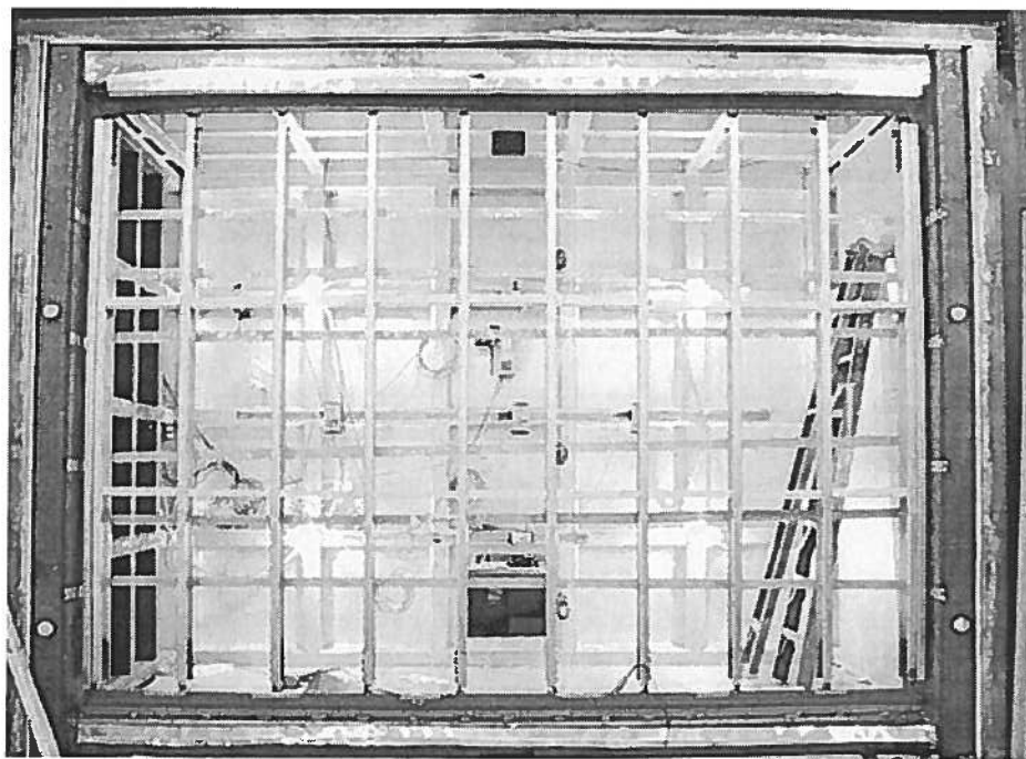
Figure 5. Typical Stud Wall Test Set-Up
