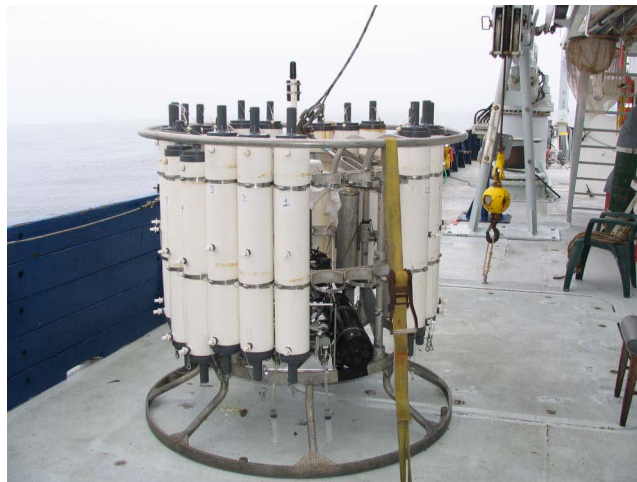
Figure 4. The CTD frame with TAPS and a fluorometer was used to measure the vertical distribution of phytoplankton and zooplankton.
