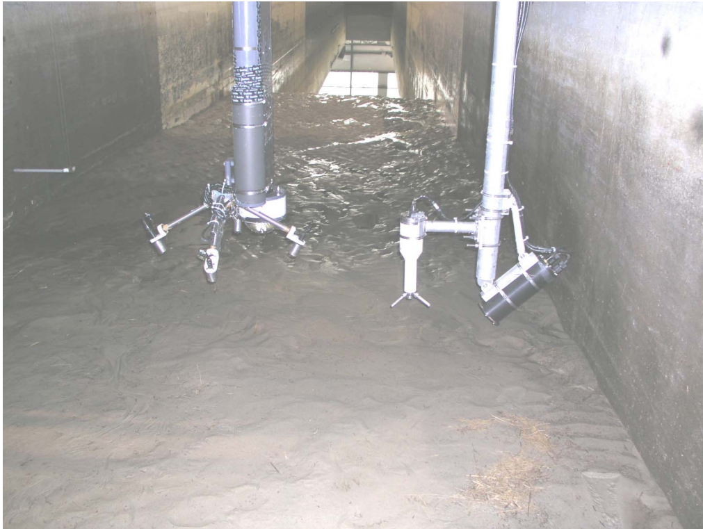
Figure 1. A view of deployed instruments looking down the sand beach (at “low tide”) within the OSU Large wave Flume during CROSSTEX. The left spar supported the 5 beam BCDV velocity and suspended sediment profiler, the acoustic scanned altimeter, and the scanned laser. The right spar suspended a reference ADV current sensor and camera that imaged the bedforms and scanned laser patterns.
