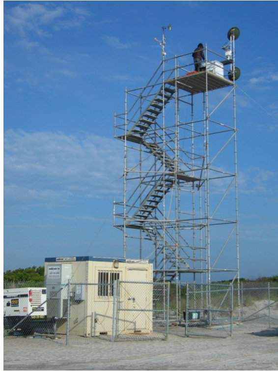
Figure C3: CORAR was deployed on the south bank of the inlet (34.529695, -77.344419). The antennas were on top of scaffolding at a height of around 12 m above the water.
