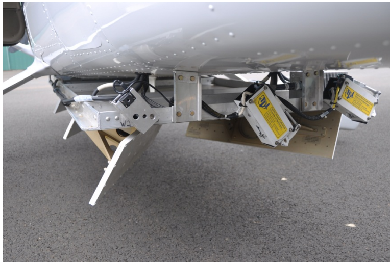
Figure C1: microASAR antennas and IR/visible cameras installed on the belly of the Cessna 172.
