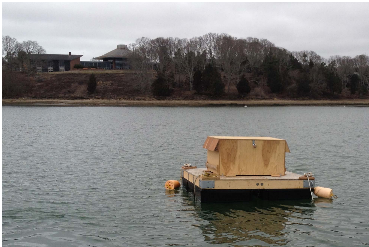
Fig. 5. Deployment of an IFCB beta unit on a cable-free mooring in Salt Pond (Nauset, MA) (Feb – June 2012). The box contains the batteries, generator, control electronics, and Ethernet radio, while the IFCB is suspended below the raft at 4 m depth. The IFCB is connected to the internet via a radio link in the Salt Pond Visitor Center (in background).
