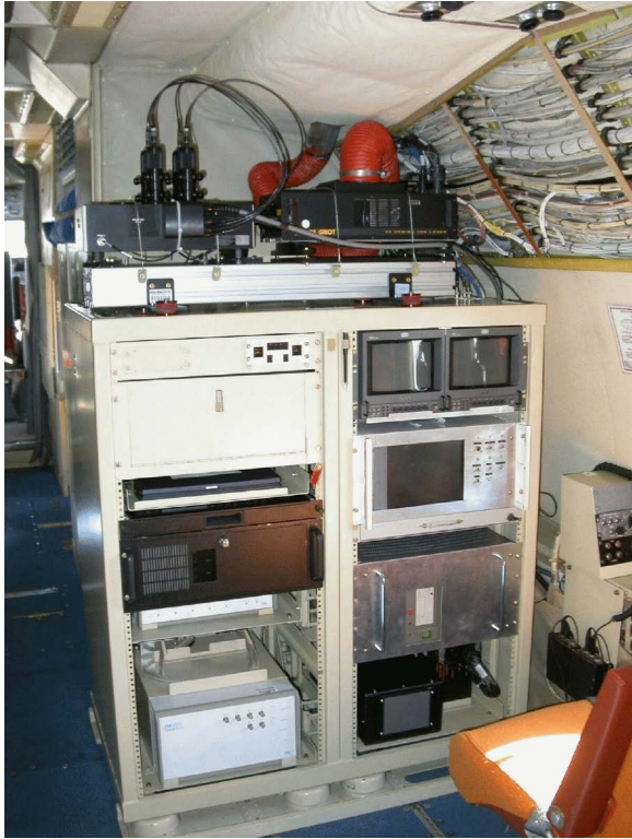
Figure 1: Photographs showing the installation of the phase-Doppler anemometer on the NOAA P-3 N43RF (Miss Piggy). Left image shows electronics (beige box in lowest left shelf of rack, laser power supply and frequency converter (black boxes in lowest right shelf), data acquisition computer (notebook computer on tray in the middle of the rack on the left side), and laser and fiber optic coupler (black boxes mounted on aluminum rail on top of the rack) as mounted in the rack at station C3X. The right image shows the transmitting (lower cylindrical object on vertical mounting post) and receiving optics (upper cylinder on post) mounted to look out the window at station C7.
