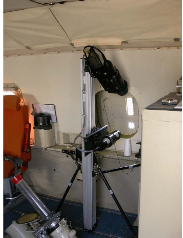
Figure 1: Photographs showing the installation of the phase-Doppler anemometer on the NOAA P-3 N43RF (Miss Piggy). Left image shows electronics (beige box in lowest left shelf of rack, laser power supply and frequency converter (black boxes in lowest right shelf), data acquisition computer (notebook computer on tray in the middle of the rack on the left side), and laser and fiber optic coupler (black boxes mounted on aluminum rail on top of the rack) as mounted in the rack at station C3X. The right image shows the transmitting (lower cylindrical object on vertical mounting post) and receiving optics (upper cylinder on post) mounted to look out the window at station C7.
