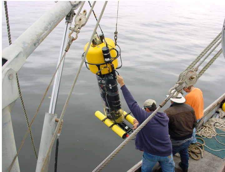
Figure 1. URI Scientists deploying the IOPC profiler with the newly developed APNA II nutrient analyzer payload in Monterey Bay from the R/V Shana Rae.
