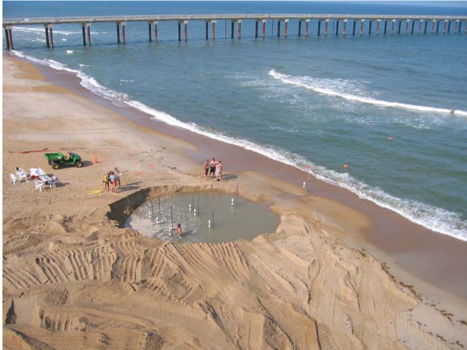
Figure 2. [Overhead photograph of a 10-m diameter, 2-m deep hole created with heavy equipment near the low-tide shoreline. Ten sensors with colocated pressure gages and current meters (white cylinders) were used to measure flows and waves in and offshore of the hole at mid to high tide levels. The surrounding sand levels were surveyed continuously as the hole filled in with sediment.]
